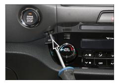
1. Remove screws of OEM head unit (left and right)
