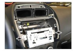
2. Remove OEM Radio/CD device
