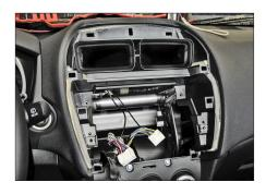
3. Dashboard with removed OEM Radio/CD device
