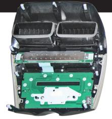
4. Dismount air vents left and right. Remove OEM circuit board (PCB).
