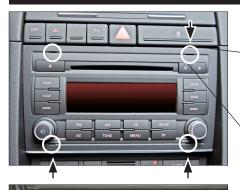
Put four radio release keys in the appropiate slots of the OEM radio
