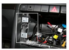
Place mounting frames as positioning help in order to to be cut away
