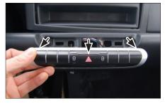
Remove the switch unit (fixed by clamps) by pulling it towards you
