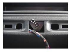
Remove the TORX TX25 screw holding the surrounding frame (see arrow)
