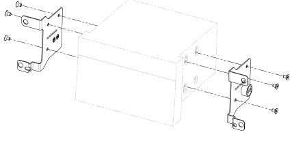
5. Mount mounting brackets left and right to INE-W928R Connect all required circuit points and place the Double DIN head unit on dash board
